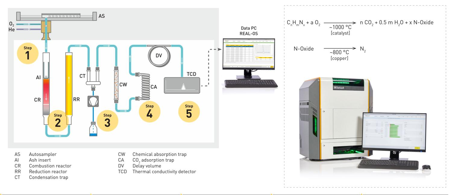
The sample enters the Dumas system via autosampler (AS). In the combustion reactor (CR) at temperatures from approx. 1000°C an exothermic reaction takes place between oxygen (02), the tin foil and the sample. The sample is completely combusted with the help of oxidation catalysts.
