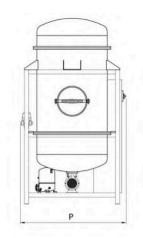
Vacuum evaporator to treat water-based solution from 10 to 750 L/h. Recommended for medium quantitative of wastewater.
