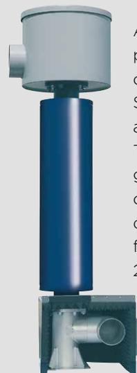
A specific kit for Robox packages in vacuum operation, consisting of SDL absorption silencers and SPS exhaust silencers. This reduces the sound level generated by the exhaust outlet by approximately 25 dB(A) within the frequency field ranging from 200 Hz to 20 kHz.
