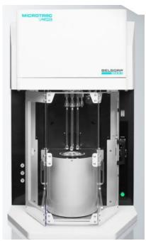
The <u>BELSORP MAX II</u> is used to evaluate the BET specific surface area and pore size distribution of various solid materials such as powders, fibers, membranes by gas adsorption/vapour.
