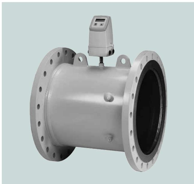
The 2-track flowmeter SITRANS FUS380 comes as battery or mains-powered and is designed to measure water flow in district heating plants, local networks, boiler stations, substations, chiller plants and other general water applications.
