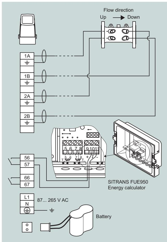
The scheme shows the transducer cable connections between transmitter terminals and respective transducer and the electrical connection of the energy calculator SITRANS FUE950.
