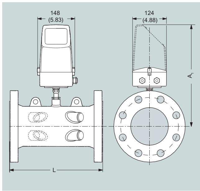
Transmitter IP67/NEMA 4X/6, wall mounting
