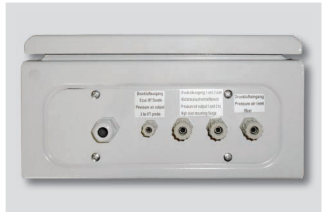
Connections for the cleaning unit.
