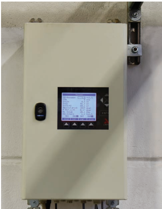
LT2K with integrated reference air pump.
