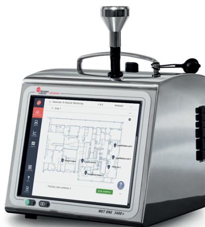
Figure 3. The MET ONE 3400+ with on-screen interactive Routine Environmental Monitoring map
