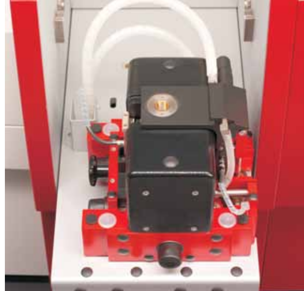
▲ Graphite furnace in service position
