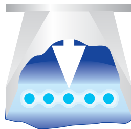
High flow rate + poor water quality = more intense UV radiation
