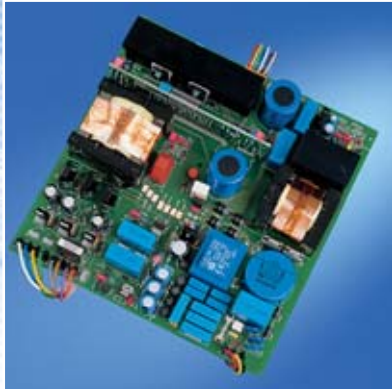
Electronic ballasts ensure that the Spekthrotherm® UV lamps operate cost-effectively and reliably
