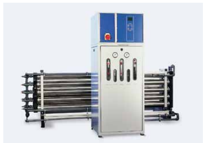
INDUSTRIAL SCALE 2-STAGE REVERSE OSMOSIS EQUIPMENT.
