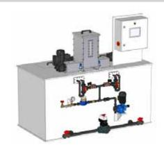
The tank of the batch system consists of 2 separate chambers. The polymer solution is prepared successively in the chambers. After a defined maturing time, the polymer solution can be used. Product carryover is ruled out.
