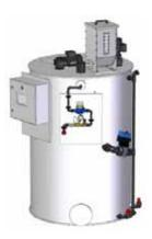
In the case of the double decker variant, the chambers are installed one above the other. Preparation of the polymer is effected in the top chamber. The matured product is drained into the lower chamber after the maturing time has ended. Because of this process, a product carryover is prevented.
