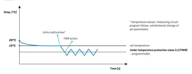
Under temperature protection class 3.2 to DIN 12880 is a standard function for CHL PREM TOP+ version and optional for CHL BASIC, COMF, PREM; ZL COMF and PREM models.
