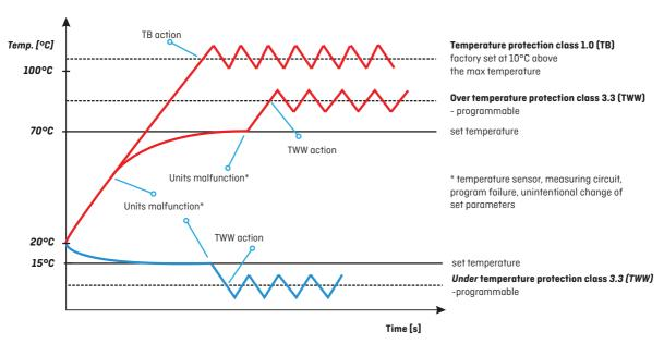
Over/under temperature protection class 3.3 to DIN 12880 is a standard function for the KK, ST PREM TOP+ and IL in the TOP+ version. It is an additional option for ST BASIC, COMF, PREM and IL in the STD version.
