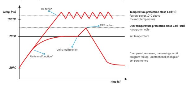
Over temperature protection class. 1.0 to DIN 12880 is a standard function for the ST/CHL/CL/IL/SR/KK equipment. It is factory set at approx. 10°C above the max temperature. Over temperature protection class 2.0 to DIN 12880 is a standard function for the CL/IL/SL/SR equipment in the STD version and ST/CHL PREM models.
