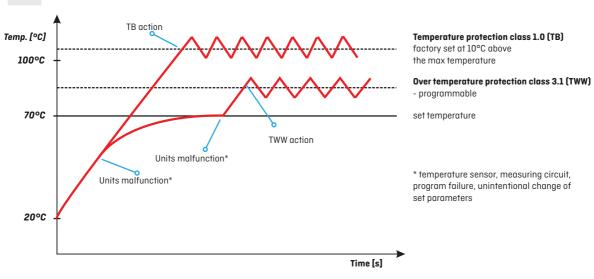
Over temperature protection class 3.1 to DIN 12880 is a standard function for the CL/SL equipment in the TOP+ version, and optional for the CL/SL/SR ranges in the STD version.
