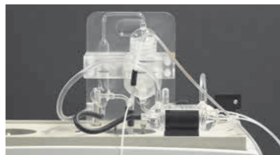
Simple or double in-line distillation for measurement of Phenol Index and Cyanides in water.
