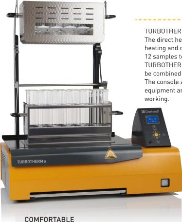
TURBOTHERM is a digestion unit based on infrared technology. The direct heat input by infrared radiation provides short heating and cooling times: Only 10 minutes are needed to bring 12 samples to boil.
