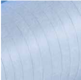
Endless fiber structure limits fiber migration at a bare minimum
