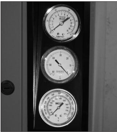
Discharge pressure, filter restriction, and temperature gauges are standard.
