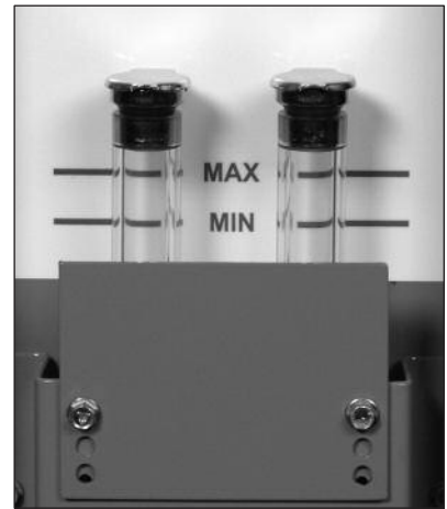
Oil fill level site glass.
