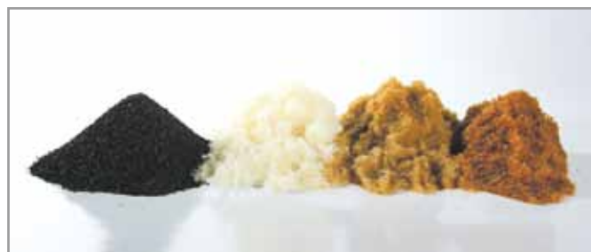
ACTIVATED CARBON, ANIONS, MIXED BED AND CATION EXCHANGE RESINS (FROM LEFT TO RIGHT)
