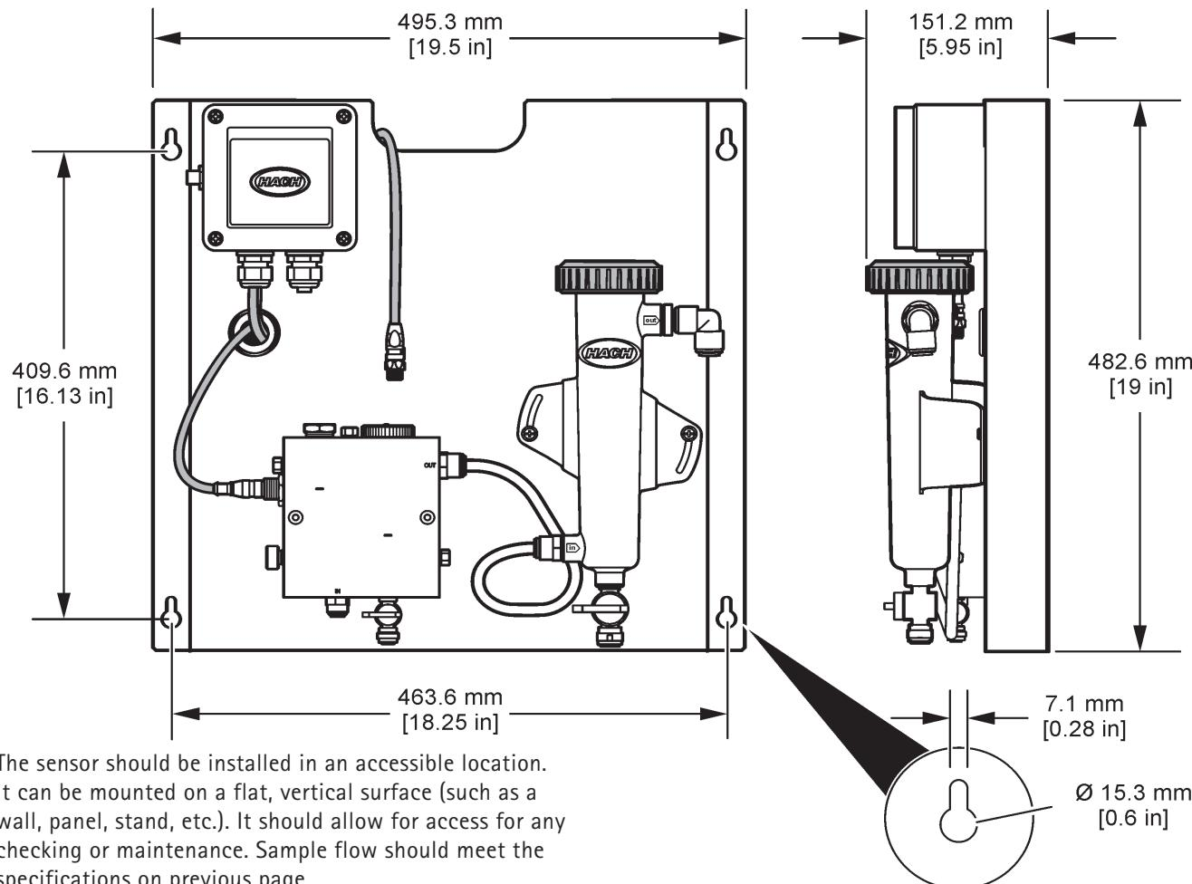
The sensor should be installed in an accessible location. It can be mounted on a flat, vertical surface (such as a wall, panel, stand, etc.). It should allow for access for any checking or maintenance. Sample flow should meet the specifications on previous page.
