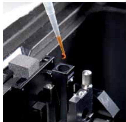
Adjustable cell holder with ultra-micro cell for precise quantitative analysis of extremely small sample volumes
