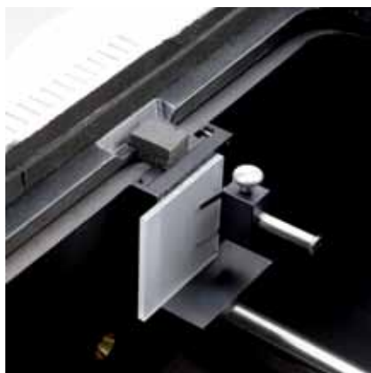
Solid sample holder to determine transmission characteristics
