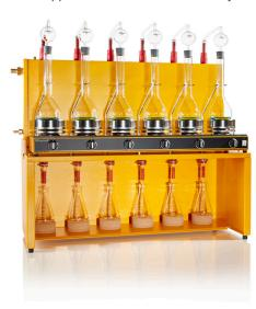
For Kjeldahl flasks of sizes 50, 100, 250, 500 and 750 ml. Each heater can be adjusted individually and continuously. With Kjeldahl flasks, Reitmair tops, condenser tubes, discharge tubes, Erlenmeyer flasks, all rubber connectors, stands and mains cable.
