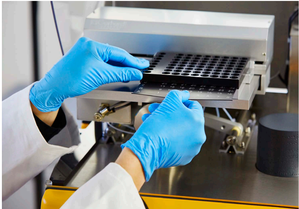
Exact positioning – precise traceability: all samples have preset positions.
